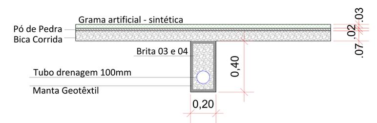
2 DETALHE CORTE VALA DE DRENAGEM ESC: 1/25
