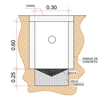
6 DETALHE CORTE SUMIDOURO ESC: 1/25
